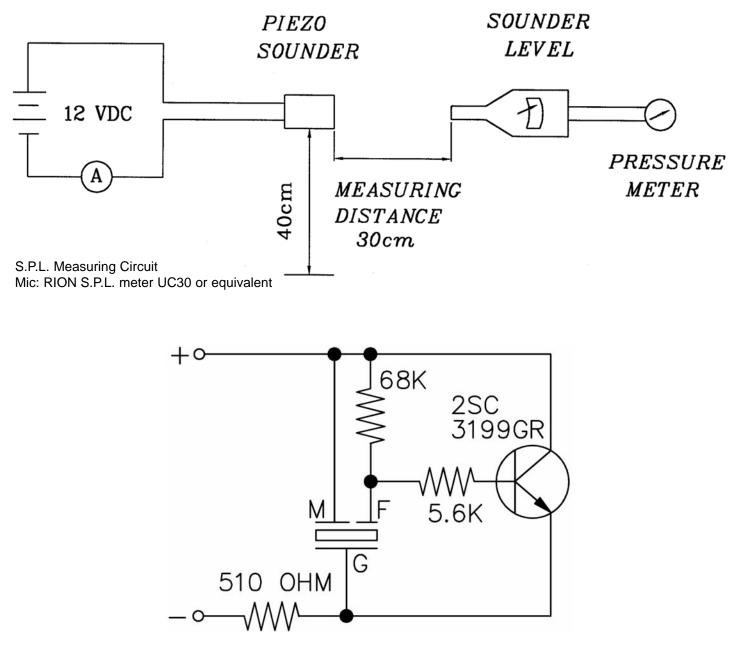
The current consumption and the sound pressure level are measured by using the recommended driving circuit shown above.
